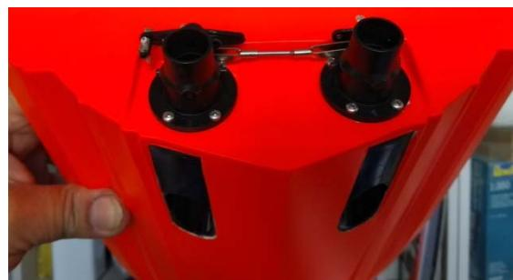
Now also mount the reverse flaps of the jet and connect them to the two front servos. Check the function of the steering and the reverse flaps accurately.
