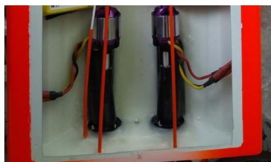
Then the shafts with couplings and the engines are installed and the jet end piece is screwed through the hull.
