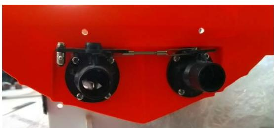
Mount the connecting rod between the two steering levers and adjust it so that the jets are exactly parallel.
