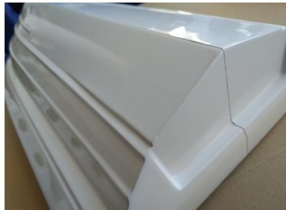
Drill as many small holes as possible within the markings, especially in the corners and radii, between which you then cut out the cut-outs with a mini cutting disc and files.
