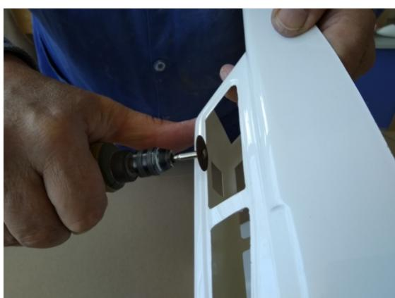
The cabin housing (5) is now drilled out within the thin window markings and cut and filed down to the markings.
