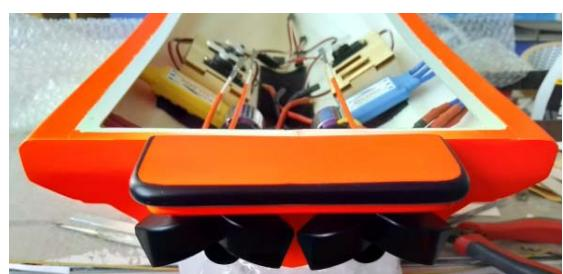
We recommend that you prepare everything for mounting the remote control and battery according to your own measurements before gluing on the deck (2).
