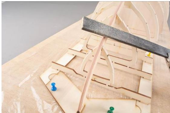
Fig.: Bevelling keel battens and frames
