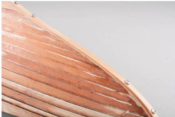
Fig.: Strips glued on
