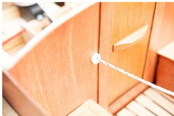
Fig.: Sheet lead-through mainsheet
