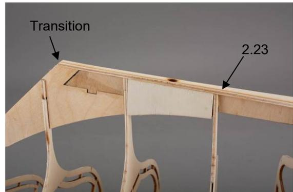
Fig.: Aligning and gluing on the keelson, keel bolt at the rear
