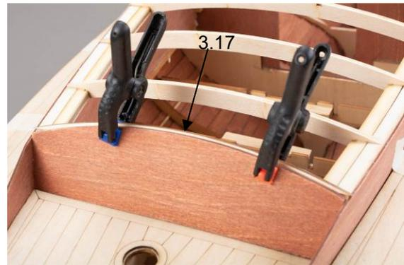
Fig.: Gluing in the roof frame
