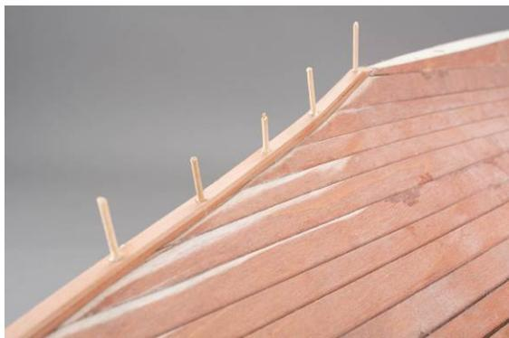
Fig.: Closing the screw holes
