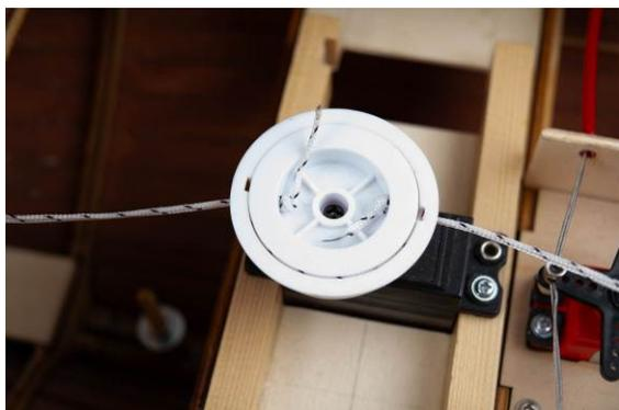
Fig.: Sail winch installed
