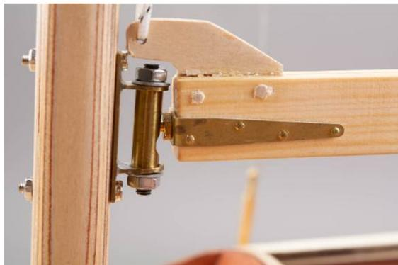
Fig.: Boom fitting complete (will be attached to the mast later)
