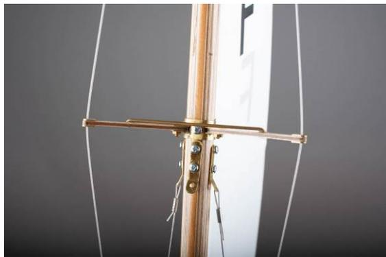
Fig.: spreader and shroud or jib attachment
