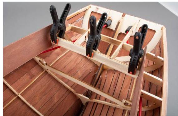
Fig.: Gluing in the doubling
