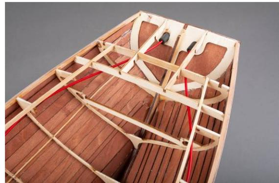
Fig.: Bowden cable tube
