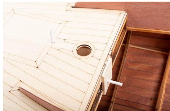
Fig.: Gluing in the sheet guide (here installed in the prototype with extra boards, no longer necessary)
