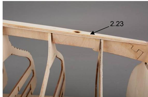
Fig.: Aligning and gluing on the keelson, keel bolt at the front
