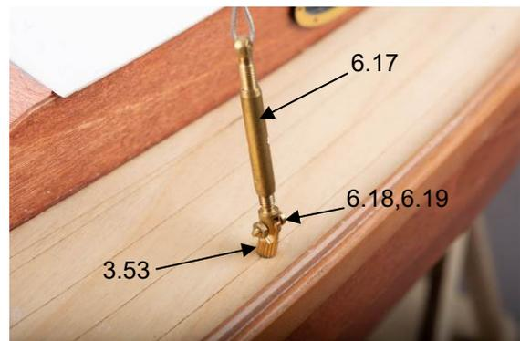
Fig.: Eyebolt and shroud tensioner
