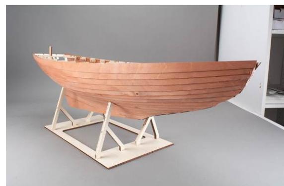
Fig.: Planked hull
