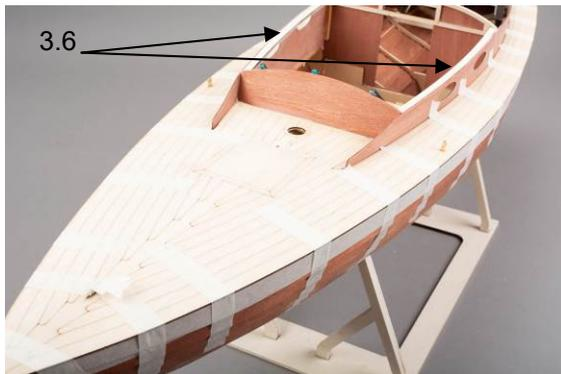
Fig.: Attaching the deck
