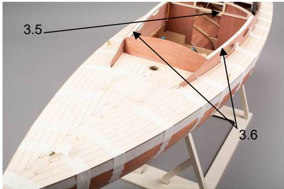
Fig.: Gluing in the roof frame
