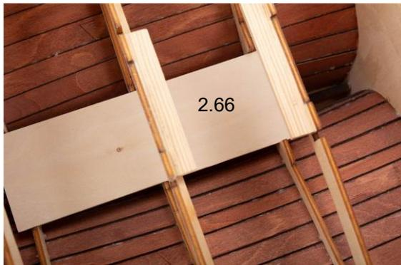
Fig.: Battery board
