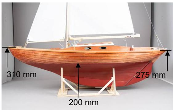
Fig.: Position for waterline
