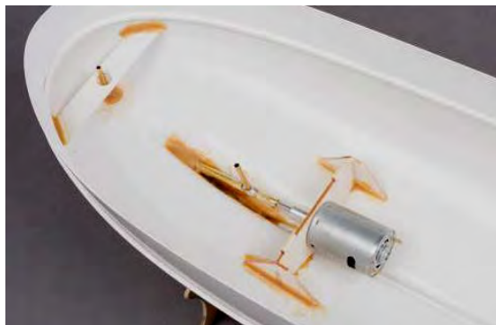
Fig. drive glued in hull
