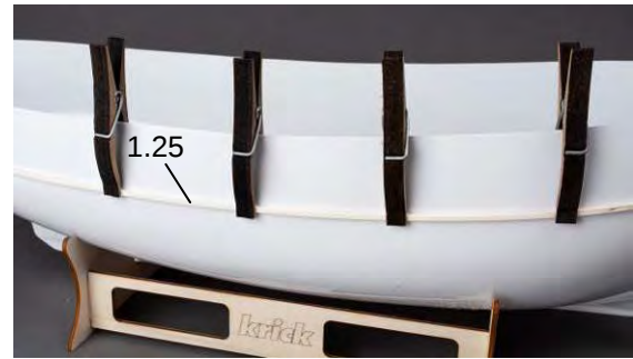
Fix the rubbing strip with clamps.
