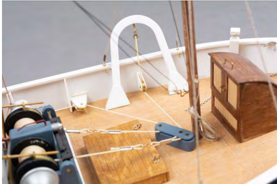
Fig. net gallows and roller blocks
