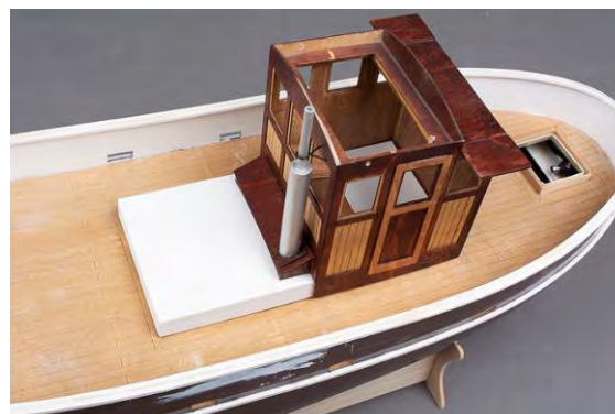
Fig. Position the superstructure on the hull
