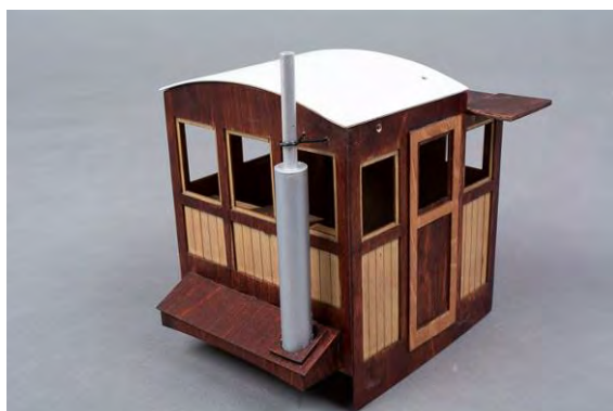
Fig. superstructure with exhaust pipe
