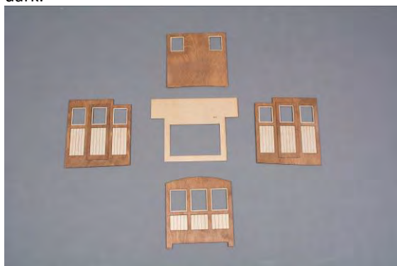
Fig. superstructure parts stained and glued
