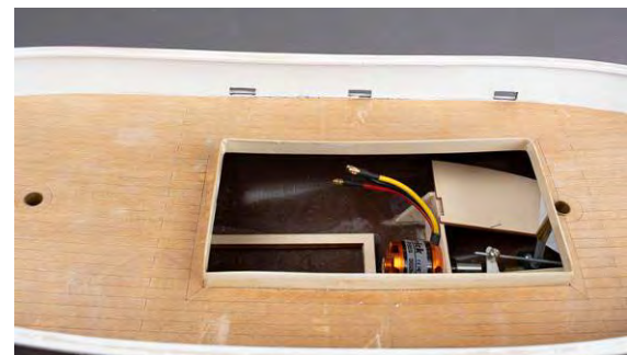
Fig. scuppers made and deck placed
