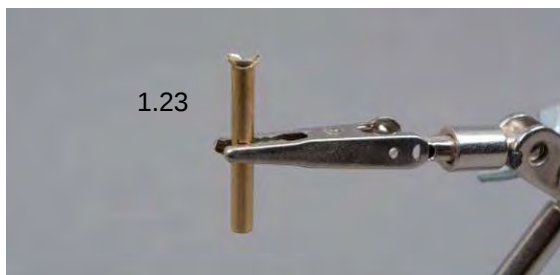
Fig. lubrication nipple with notch
